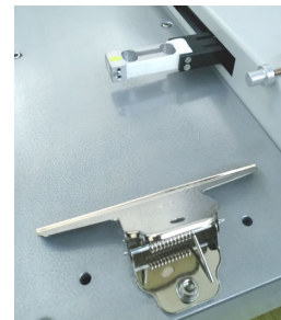
Customized Clamp for low COF material
